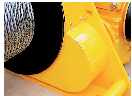
Parti meccaniche protette. Safety: mechanical parts are protected.
